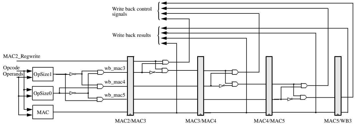
**Figure 2. Implementation of the variable latency (2 to 5 cycles) MAC pipeline.**
