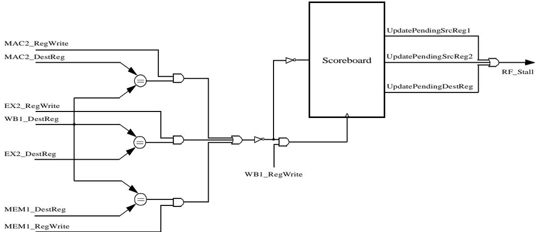
**Figure 3. Control logic for scoreboard update from WB1.**
