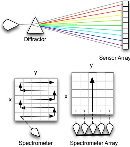
**Fig. 2.** *Hyperspectral imager architectures.* Top: A spectrometer consists of a diffractor (grating or prism) and a sensor array that records light intensities at a variety of wavelengths. Bottom: Whiskbroom designs move the spectrometer spatially throughout the image, scanning one location at a time. Pushbroom designs scan the image along a spatial direction using a spectrometer array.
