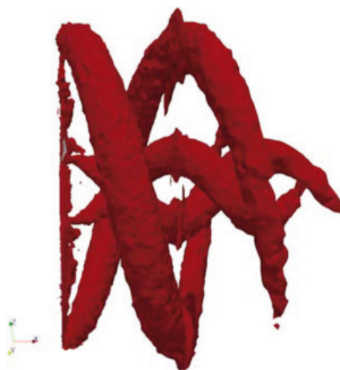
Figure 14. Iso-surface of the second invariant velocity gradient tensor at Q = 0.3 \text{ 1/s}^2 , for the 10 m/s case. This identifies the trailing vortices at the tip and the root
