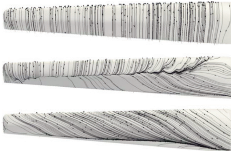
Figure 12. Limiting streamlines on the suction side of the blade for the inlet velocity of 5 m/s, 10 m/s and 21 m/s
