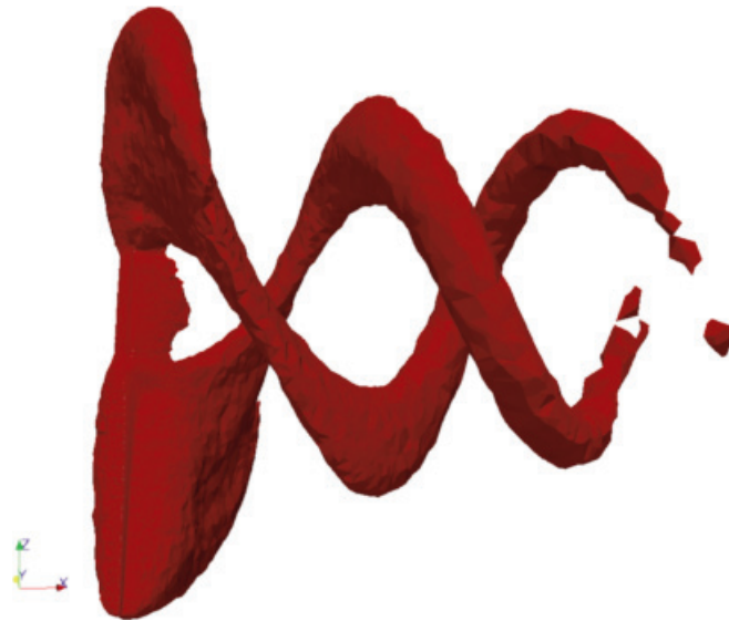
Figure 15. Iso-surface of X velocity at U_x = 8.1 m/s, for the 10 m/s case
