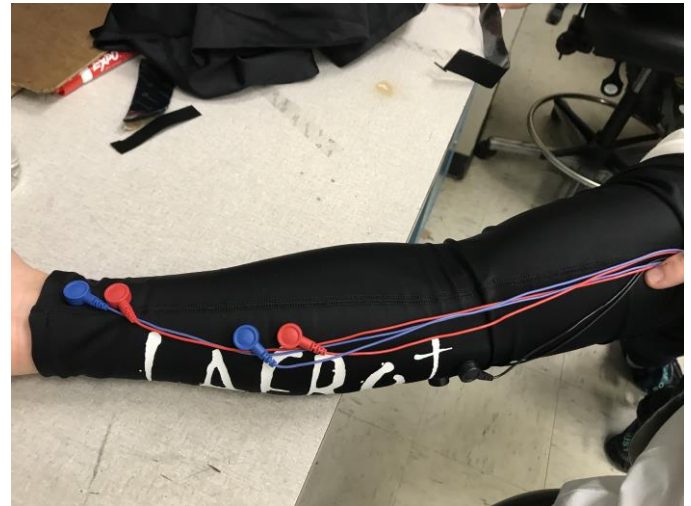
Figure 15: Custom EMG Electrode Sleeve Prototype.
