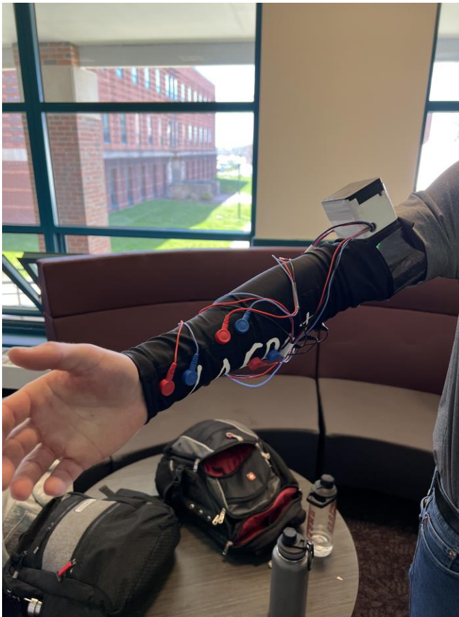
Figure 6: Final prototype of EMG electrode sleeve with enclosed PCB strapped onto bicep using Velcro.
