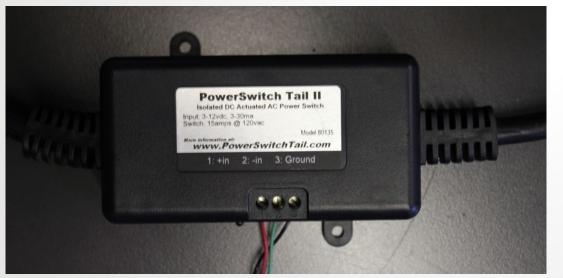
Specification: 5V input Switching 120VAC *How to wire:* Power -> +in Signal -> -in Gnd -> Ground
