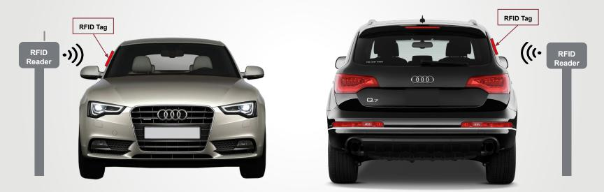
Represented above are the different entry and exit points of a parking lot. An RFID Reader installed at this location will detect RFID tags, embedded in the UMass Parking Stickers in vehicles entering/exiting to activate a clock timer accordingly, which will calculate the cost. Users will not have to stop at the entry point to generate a ticket or be required to pay for parking manually.
