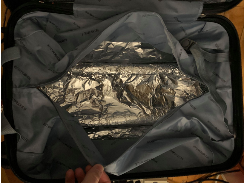
One side of the LoadOut suitcase, shielding behind the lining
