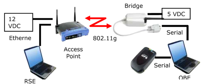
Figure 8 Connectivity of the prototype system (see online version for colours)
