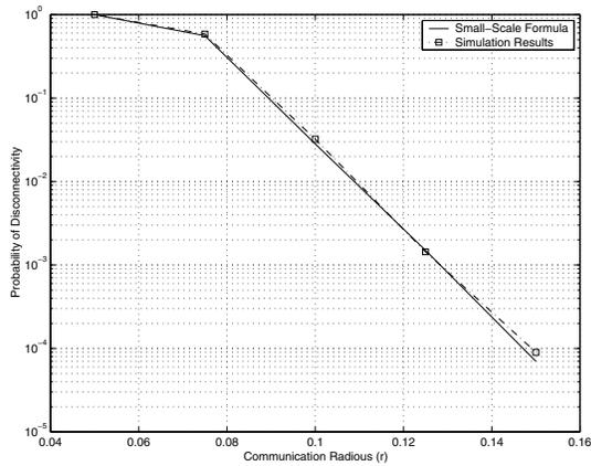
Fig. 8. Disconnectivity probability of  $g(500, r, 1)$  using (10) and simulation results.
