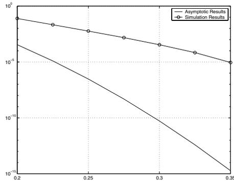
Fig. 2. Comparison of asymptotic results with the small scale simulation results for the probability of disconnectivity of  $g(n = 100, r)$ .
