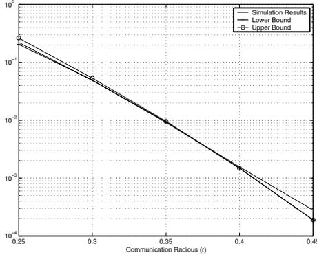
Fig. 5. Disconnection probability of  $g(100, r, .5)$ : lower bound, upper bound, and the simulation results.
