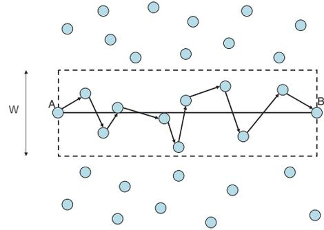
Fig. 11. Illustration of a simple geometric routing.
