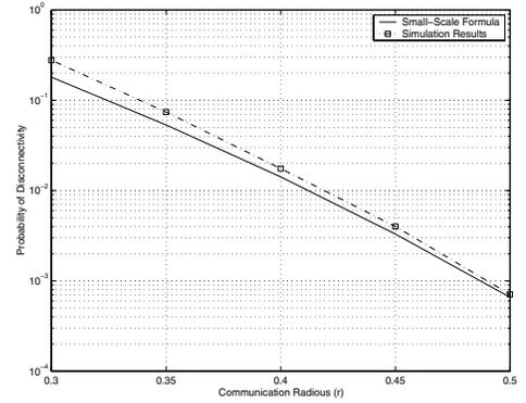
Fig. 7. Disconnection probability of  $g(30, r, 1)$  using (10) and simulation results.
