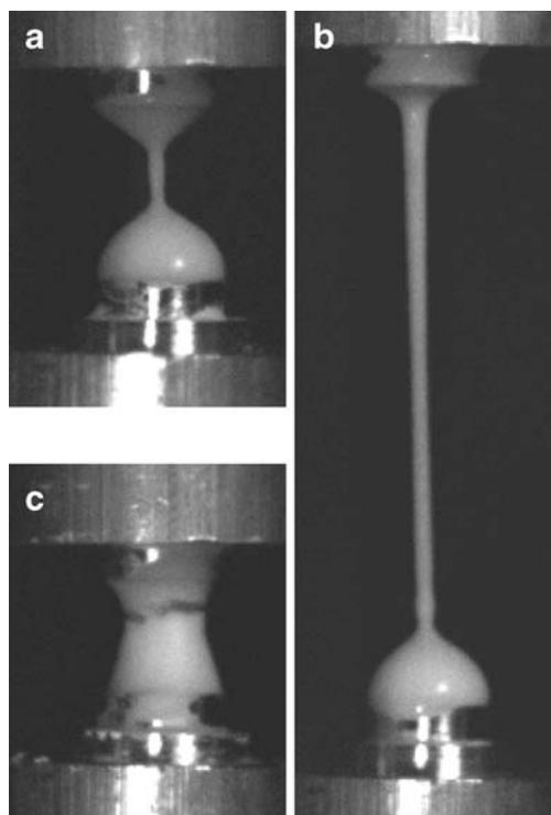
**Fig. 4** High-speed images of 55 wt.% cornstarch in water suspension being stretched. The images demonstrate **a** the Newtonian response of the fluid filament at a low extension rate of  $\dot{\epsilon} = 0.3 \text{ s}^{-1}$ , **b** the strain-hardening response at a moderate extension rate of  $\dot{\epsilon} = 0.9 \text{ s}^{-1}$ , and **c** the solid-like brittle fracture of the fluid filament at a large extension rate of  $\dot{\epsilon} = 1.5 \text{ s}^{-1}$
