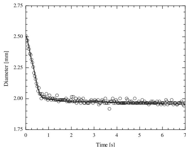
**Fig. 7** Diameter decay measurements for a CaBER measurement of a 55 wt.% cornstarch in water suspension. The spline used to fit the data and calculate the extensional viscosity, *thick line*, is superimposed on top of the experimental data,  $\circ$
