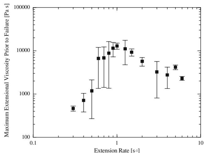
**Fig. 5** Maximum extensional viscosity achieved before filament failure for a 55 wt.% cornstarch in water suspension
