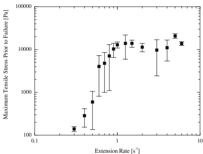
**Fig. 6** Maximum tensile stress measured before filament failure in extensional flow for a 55 wt.% cornstarch in water suspension
