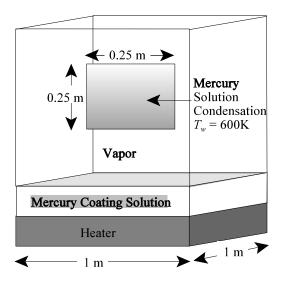
Properties Mercury Coating Solution  $T_{sat} = 630 \text{ K}$   $\rho_f = 12000 \text{ kg/m}^3$   $\rho_g = 3.9 \text{ kg/m}^3$   $\sigma = 0.42 \text{ N/m}$  (surface tension)  $k_f = 11.4 \text{ W/mK}$   $\mu_f = 9.5 \text{ x} 10^{-2} \text{ Ns/m}^2$   $c_f = 135 \text{ J/kgK}$   $h_{fg} = 295,000 \text{ J/kg}$ Pr = 1.12 Surface-Fluid Boiling Coefficients  $C_{s,f} = 0.01$ n = 1.7
