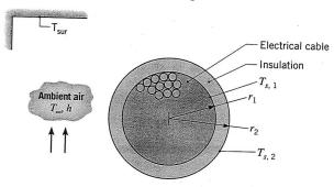
(a) Write the steady-state forms of the heat diffusion equation for the insulation and the cable. Verify that these equations are satisfied by the following temperature distributions:
