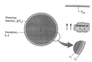
(a) Write the steady-state form of the heat diffusion equation for the insulation. Verify that this equation is satisfied by the temperature distribution
