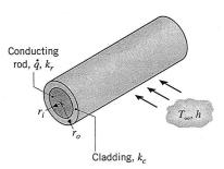
For steady-state conditions, write appropriate forms of the heat equations for the rod and cladding. Express appropriate boundary conditions for the solution of these equations.
