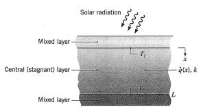
(a) Obtain expressions for the rate at which heat is transferred per unit area from the lower mixed layer to the central layer and from the central layer to the upper mixed layer.
