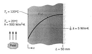
(a) Applying an overall energy balance to the wall, calculate the internal energy generation rate,  $\dot{q}$ .
