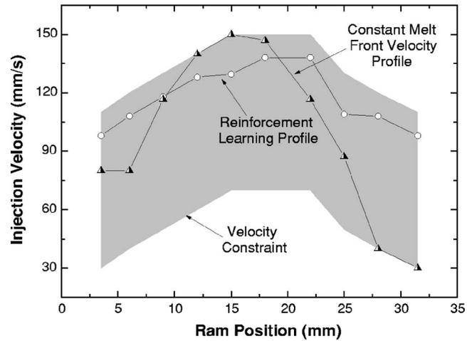
**Fig. 5 Velocity profile to maintain a constant melt front velocity compared to the one from reinforcement learning**
