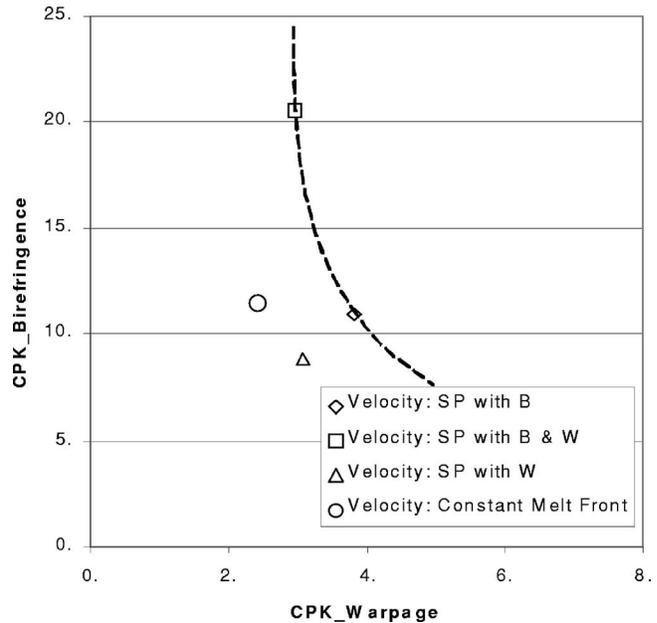
Fig. 7 Process capability of birefringence and warpage for four velocity profiles (SP refers to profiles generated by sequential programming)
