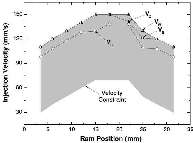
**Fig. 4 Velocity profile by sequential programming (SP) to enhance birefringence ( $V_B$ ), warpage ( $V_W$ ), and birefringence and warpage together ( $V_C$ ) compared to the profile from reinforcement learning ( $V_R$ )**
