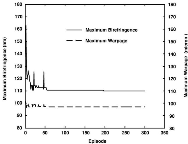
Fig. 2 Simulated values of birefringence and warpage during the adaptation of the velocity profile by reinforcement learning
