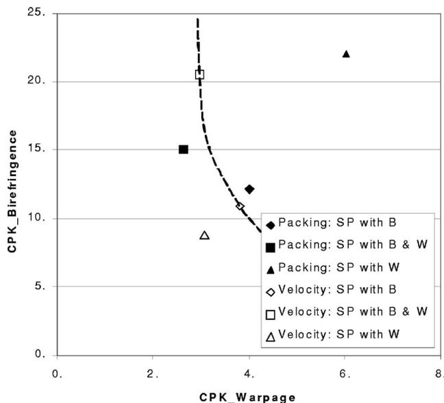
**Fig. 8 Process capability of birefringence and warpage for three pressure profiles from sequential programming (SP), along with those for velocity profiles in Fig. 7**
