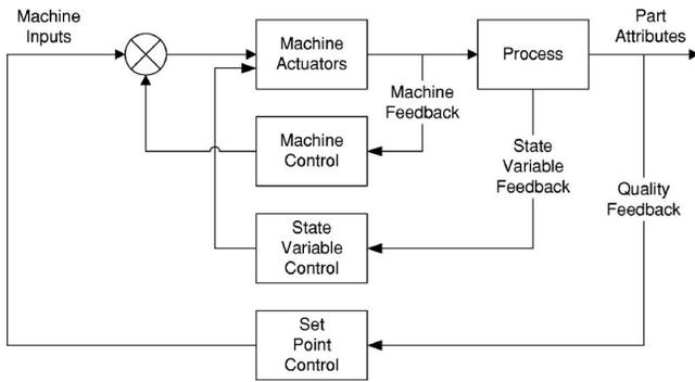
Fig. 1 Schematic of injection molding control
