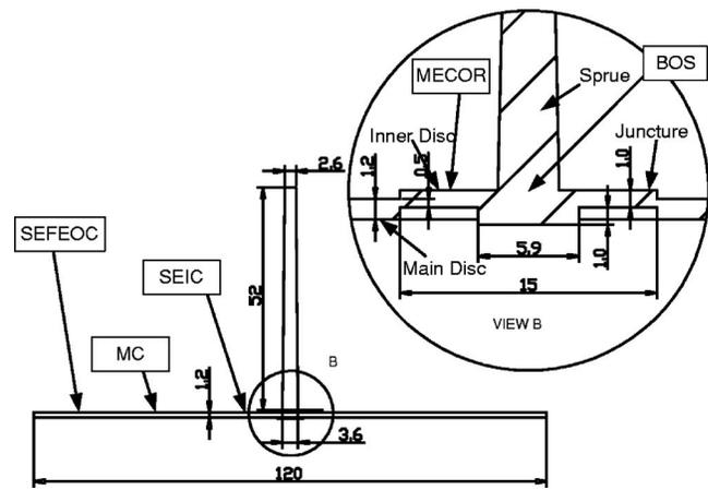
Fig. 3 Location of the recorded internal states within the mold cavity and sprue of CD-R
