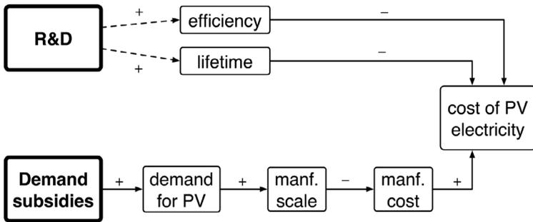
use this schema to evaluate the uncertain impact of combinations of R&D investments and subsidies on the cost of electricity over time. The central question of this paper is how R&D investment policies interact with demand subsidy policies to impact the cost of electricity from PV.
