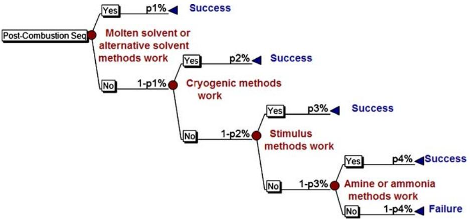
**Fig. 2** Structure of probability tree for Post-combustion
