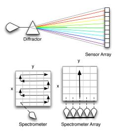
**Fig. 2.** Hyperspectral imager architectures. Top: A spectrometer consists of a diffractor (grating or prism) and a sensor array that records light intensities at a variety of wavelengths. Bottom: Whiskbroom designs move the spectrometer spatially throughout the image, scanning one location at at time. Pushbroom designs scan the image along a spatial direction using a spectrometer array.
