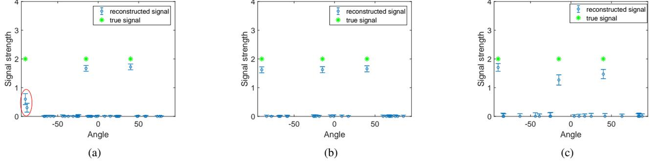
Fig. 4: Estimated signal direction and strength, SNR = 10 dB,  $N = 3, L = 100, M = 12$ . (a) Normal array with general  $\ell_1$  norm algorithm [9], (b) normal array with pairwise algorithm (III-B) and (c) cluster array with pairwise algorithm (III-B).
