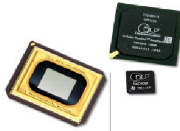
Figure 16. Discovery 1000 chipset with 0.7 XGA DDR DMD, digital controller, and analog mirror reset driver
