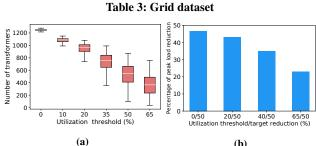
Figure 4: Selective Peak Shaving: (4a) Number of transformers whose load is shaved for different utilization thresholds, and (4b) Percentage of load reduction for different utilization thresholds.
