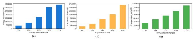
Figure 9: (9a) Impact of increased battery penetration on demand reduction, and (9b) Impact of increased EV penetration on demand reduction, and (9c) Impact of increased HVAC setpoint level on demand reduction.
