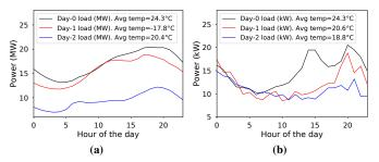
Figure 2: (2a) Power load experienced by the whole grid on three different days, and (2b) power load experienced by a transformer on three different days.
