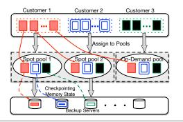
Figure 5. SpotCheck's architecture using multiple pools.
