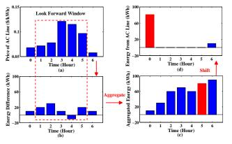
Figure 4: An example of using a look forward window to shift an energy request to a low price period to reduce cost: Energy needed from window 1-5 is shifted to window 0.
