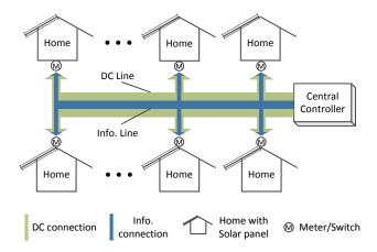
Figure 1: Architecture of Microgrids: Interconnected homes with renewable energy supply (e.g., solar panels)
