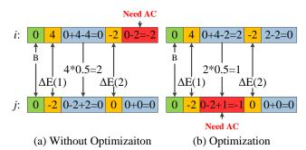
Figure 5: An example of optimization of AC allocation
