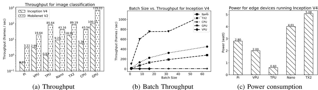
Fig. 3. (a) Throughput of edge and cloud devices for image classification. (b) The impact of batch size for edge and cloud devices for the Inception V4 model. Pi and TPU are not shown here because Pi can only run with batch size of 1 for Inception V4 model and batching for TPU is not supported. (c) Power consumption of edge devices for the Inception V4 model. The server CPU and GPU consume 131.26W and 111.66W, respectively, for the same model.
