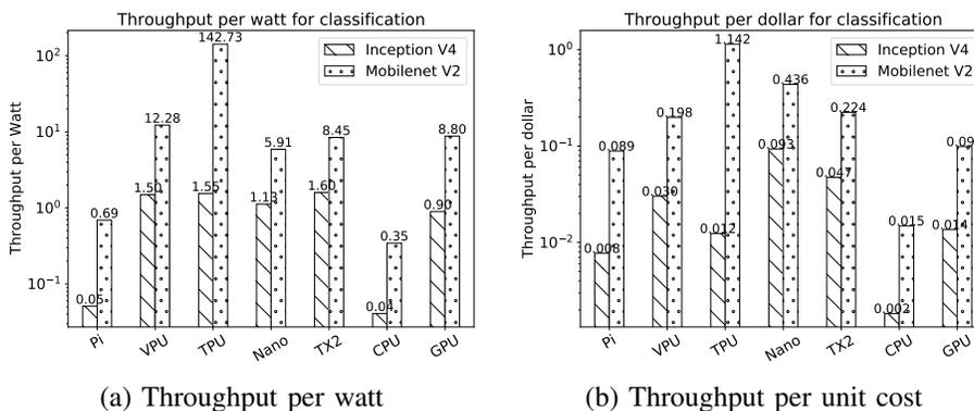
Fig. 4. Normalized performance per watt and per unit cost for various devices. Price data used for normalization is shown in Table I
