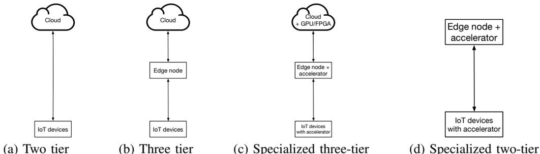
Fig. 2. Tiered architectures for IoT applications that use the device, edge, and cloud.
