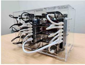
Fig. 1. A 10-node cluster of low-power Jetson nano GPUs.
