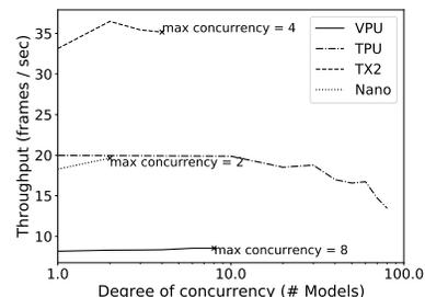
Fig. 9. Degree of concurrency supported by various device accelerators.
