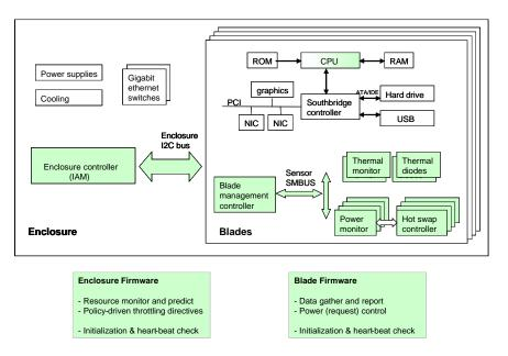
Figure 4: Implementation of enclosure-level power management.
