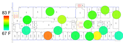
Figure 1: Variability of temperature across one floor of an office building. Ambient air temperature varies by 13°F.
