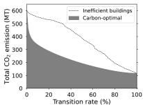
Figure 9: Carbon emissions at varying levels of electric heat pump transition while jointly optimizing for carbon emissions reduction and targeting energy inefficient buildings.
