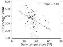
Figure 4: Relationship between energy demand of an electric heat pump and the temperature.
