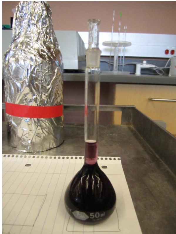
Figure 5: Photo of potassium ferrate in a buffer solution just after mixing (Martin 2011).
