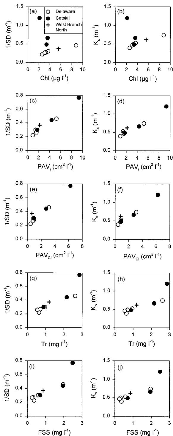
Figure 4. Analysis of roles of light attenuating constituents in regulating differences in study average conditions for optical characteristics across nine reservoir basins: (a)  $1/SD$  vs. Chl, (b)  $K_s$  vs. Chl, (c)  $1/SD$  vs.  $PAV_i$ , (d)  $K_s$  vs.  $PAV_i$ , (e)  $1/SD$  vs.  $PAV_{Cl}$ , (f)  $K_s$  vs.  $PAV_{Cl}$ , (g)  $1/SD$  vs. Tr, (h)  $K_s$  vs. Tr, (i)  $1/SD$  vs. FSS, and (j)  $K_s$  vs. FSS.
