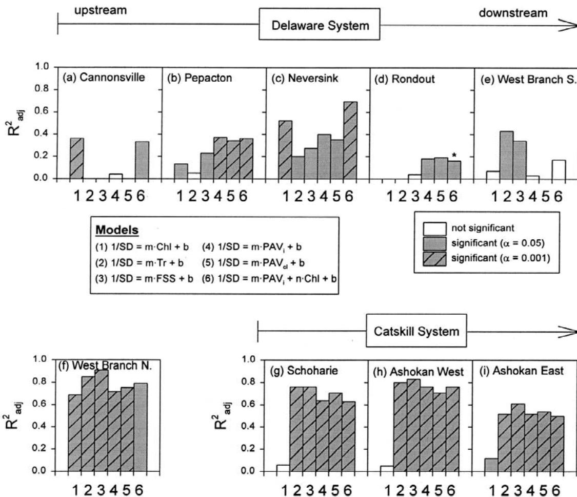
Figure 9. Performance features,  $R^2_{adj}$  and significance ( $\alpha = 0.05, 0.001$ ), of linear empirical models (see key) in predicting observed variations in  $1/SD$  for five dependent variables (individually, and Chl and  $PAV_1$  combined in multiple linear regression): (a) Cannonsville, (b) Pepacton, (c) Neversink, (d) Rondout, (e) south basin of West Branch, (f) north basin of West Branch, (g) Schoharie, (h) west basin of Ashokan, and (i) east basin of Ashokan.
