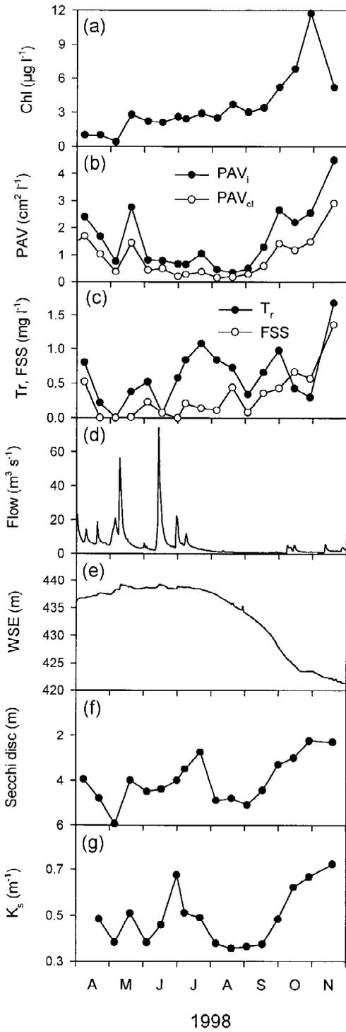
Figure 5. Time-series for Neversink Reservoir for the April–November interval of 1998: (a) Chl in the near-surface layer, (b)  $PAV_i$  and  $PAV_{Cl}$  in the near-surface layer, (c)  $Tr$  and  $FSS$  in the near-surface layer, (d) daily average flow in Neversink River, (e) daily average water surface elevation (WSE), (f) SD, and (g)  $K_s$ .
