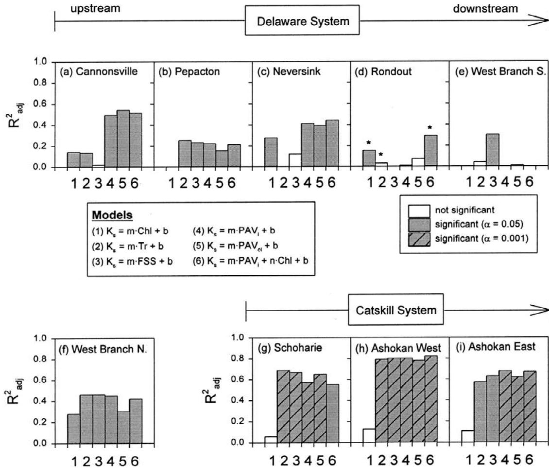
Figure 8. Performance features,  $R^2_{adj}$  and significance ( $\alpha = 0.05, 0.001$ ), of linear empirical models (see key) in predicting observed variations in  $K_s$  for five dependent variables (individually, and Chl and  $PAV_i$  combined in multiple linear regression): (a) Cannonsville, (b) Pepacton, (c) Neversink, (d) Rondout, (e) south basin of West Branch, (f) north basin of West Branch, (g) Schoharie, (h) west basin of Ashokan, and (i) east basin of Ashokan.
