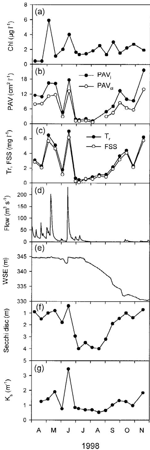
Figure 6. Time-series for Schoharie Reservoir for the April–November interval of 1998: (a) Chl in the near-surface layer, (b)  $PAV_i$  and  $PAV_{Cl}$  in the near-surface layer, (c)  $Tr$  and  $FSS$  in the near-surface layer, (d) daily average flow in Neversink River, (e) daily average water surface elevation (WSE), (f) SD, and (g)  $K_s$ .
