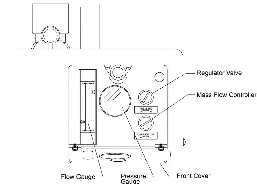
Figure 3.5 • Setting the SSM-5000A Carrier Gas Pressure
