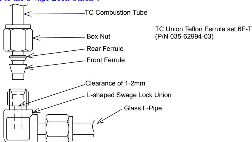
Figure 5.10 • Connecting the TC Combustion Tube to the Swage Lock Union
