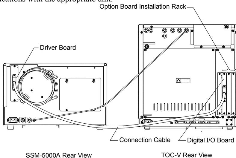
Figure 5.2 • Cable Connections of the TOC-V and SSM-5000A
