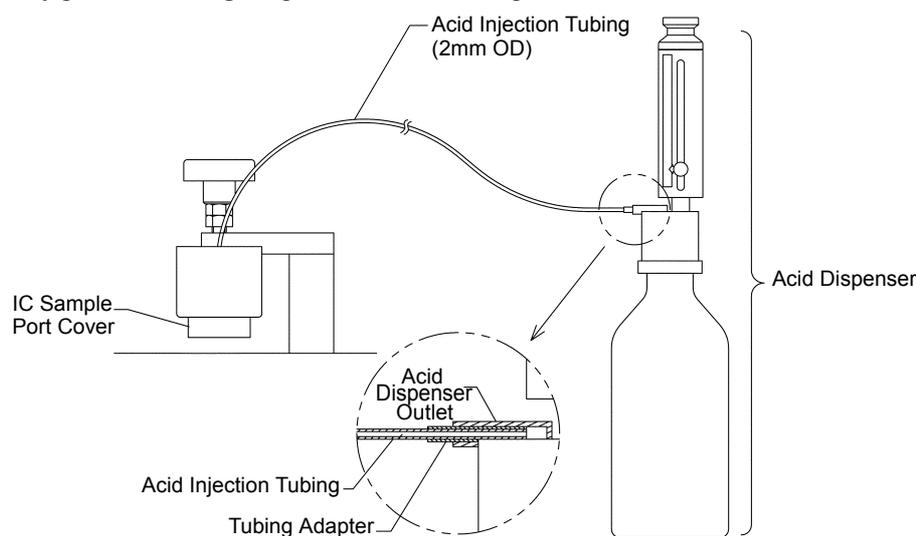
Figure 5.11 • Connecting the Acid Dispenser
