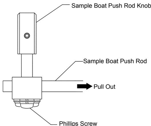
Figure 4.4 • Replacing the O-Rings - 2
