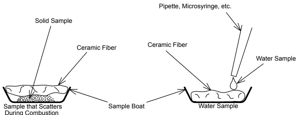
Figure 3.1 • Using the Ceramic Fiber
