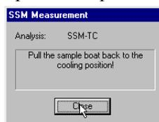
1. Return the sample boat transfer knob to the COOLING position.
