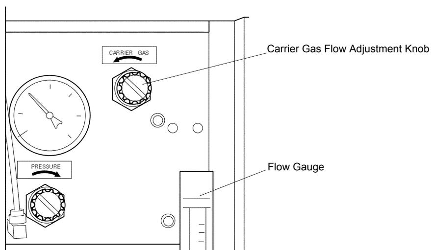
Figure 3.6 • Setting the TOC-V Carrier Gas Flow Rate
