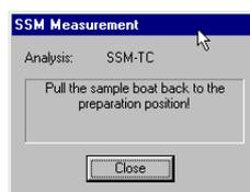
**Note:** Do not immediately return the TC furnace sample boat transfer knob to the CHANGE SAMPLE position from the MEASURING position, as this could cause damage.
