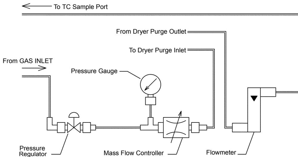
Figure 5.4 • Flow Path of the SSM-5000A Flow Controller
