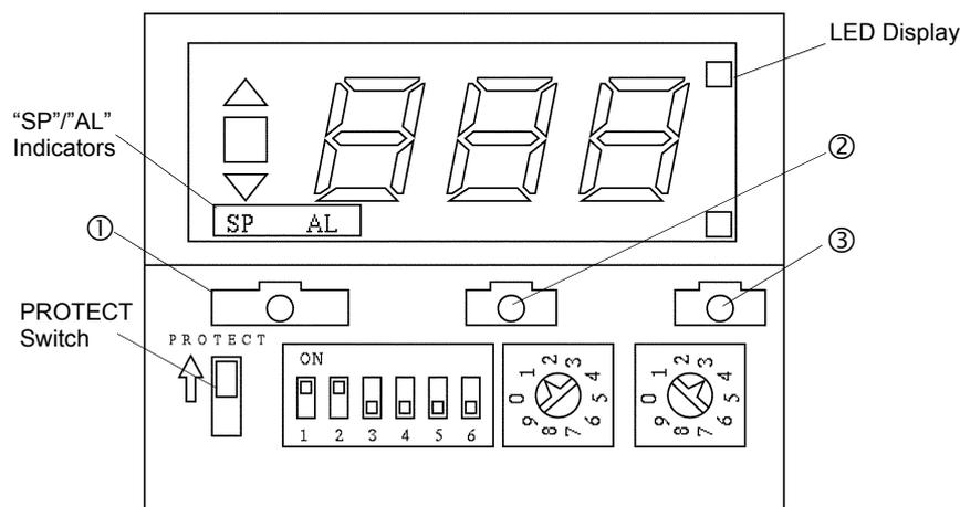
Figure 3.3 • Temperature Controller
