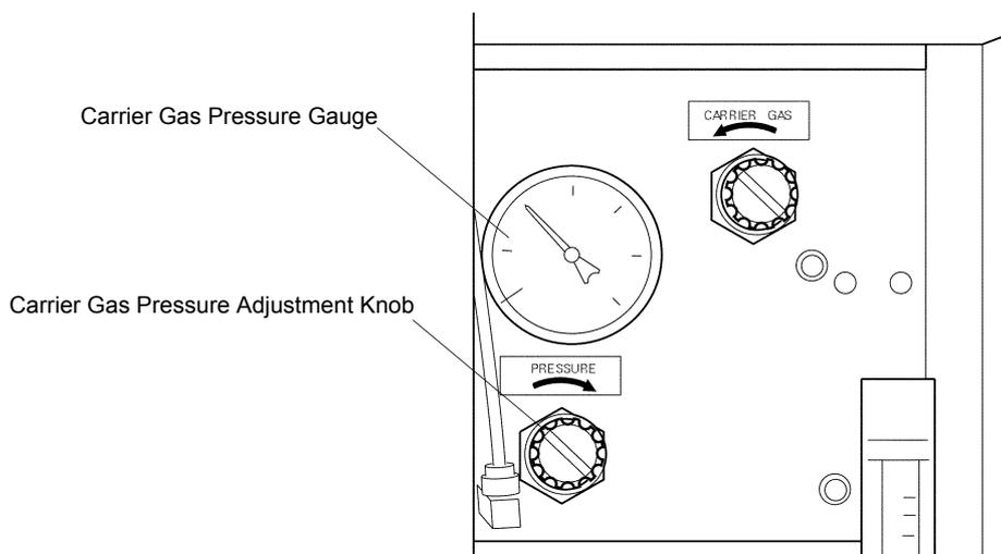
Figure 3.4 • Setting the TOC-V Carrier Gas Pressure
