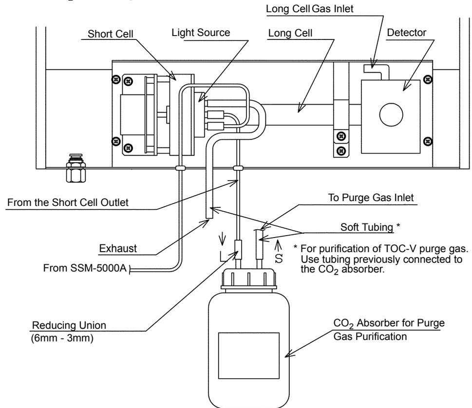
Figure 5.5 • Gas Connections to Cell
