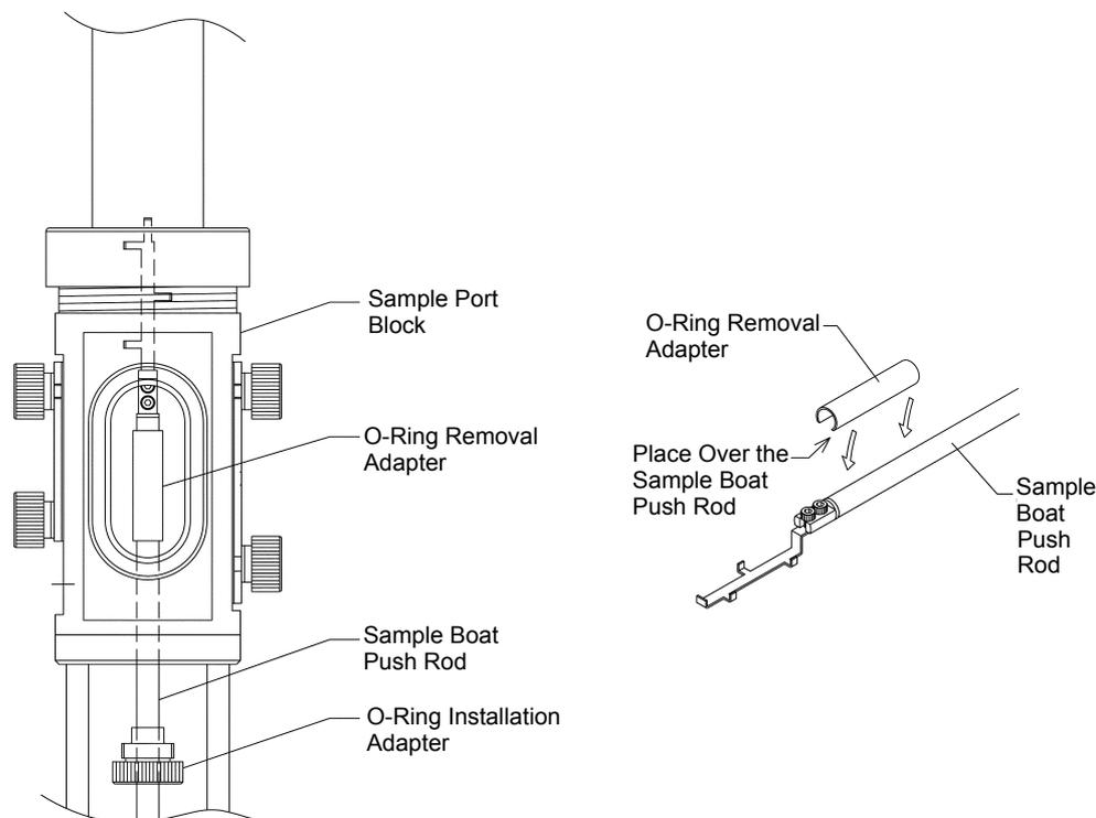
Figure 4.3 • Replacing the O-Rings - 1
