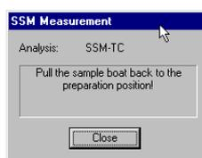
**Note:** Do not immediately return the TC furnace sample boat transfer knob to the CHANGE position from the MEASURING position, as this could cause damage.
