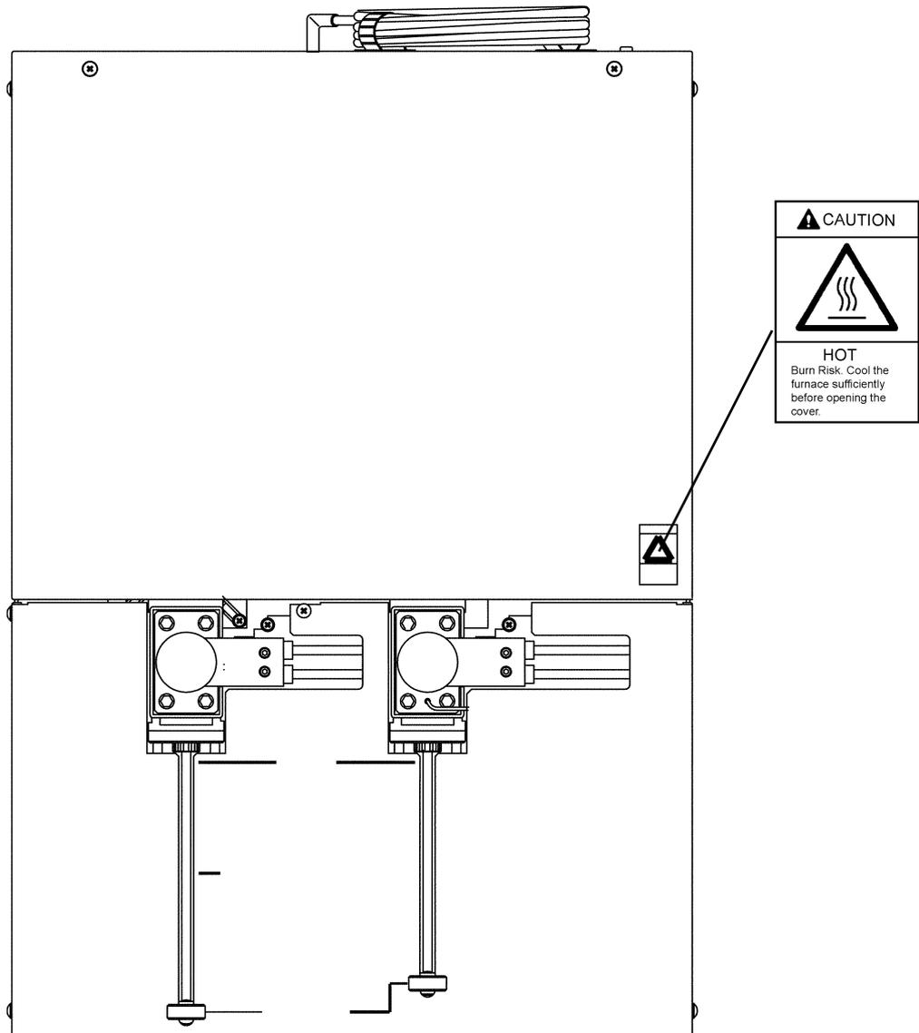
The area around the electric furnaces becomes extremely hot during furnace heating or when the furnaces reach their operating temperatures (TC furnace: 900°C, IC furnace: 200°C). Because of the danger of burn injuries, never touch these areas with bare hands. Allow the furnaces to cool before conducting maintenance on the combustion tube or catalyst.
