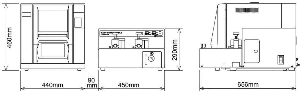
Figure 5.1 • TOC-V + SSM-5000A External Dimensions (Example: TOC-VcSH)
