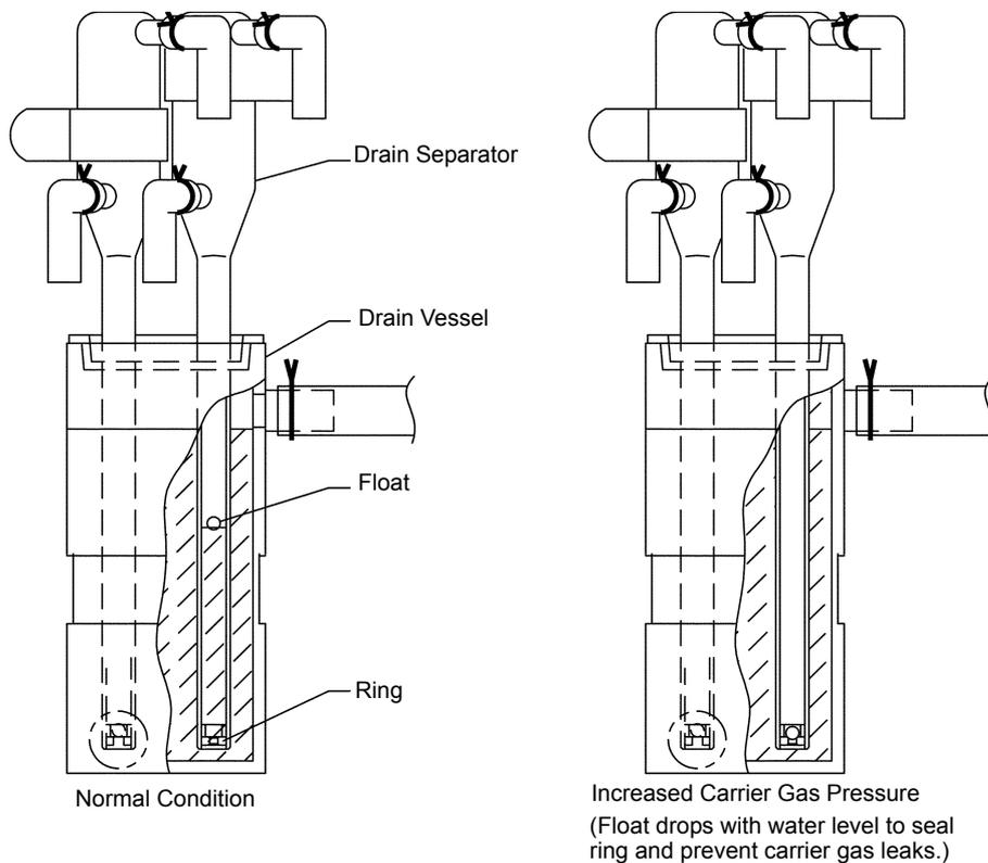
Figure 4.2 • Drain Separator
