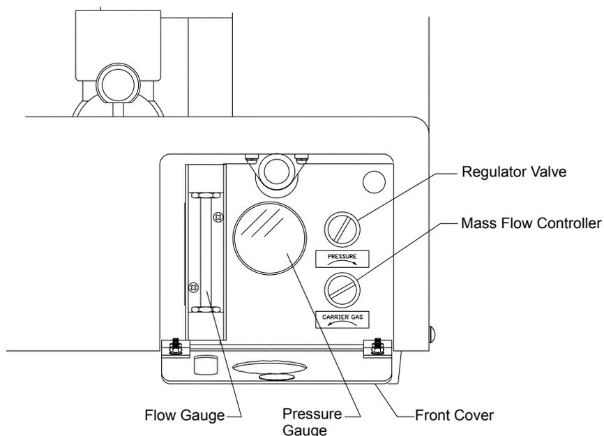
Figure 3.7 • Setting the SSM-5000A Carrier Gas Flow Rate
