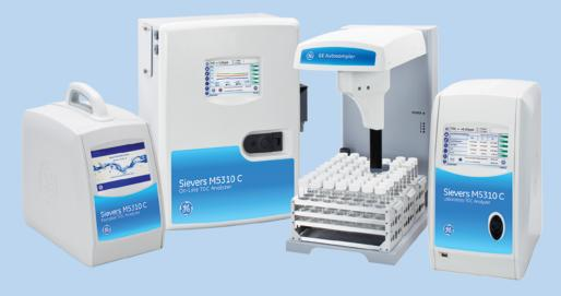
GE's Analytical Instruments Sievers\* M5310 C TOC Analyzers are designed specifically for the drinking water industry. Monitoring organic matter at drinking water treatment facilities can help plant operators understand changes in water quality and make informed decisions about treatment processes. Designed to minimize operator intervention, the M5310 C Analyzers offer cost-effective, reliable measurements—enabling process optimization and regulation compliance with ease.
