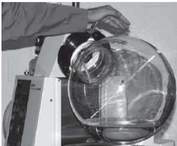
Fig. 13: Closing the snap flange coupling
