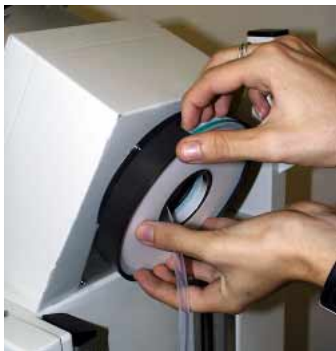
Fig. 26: Removing the evaporating flask seal
