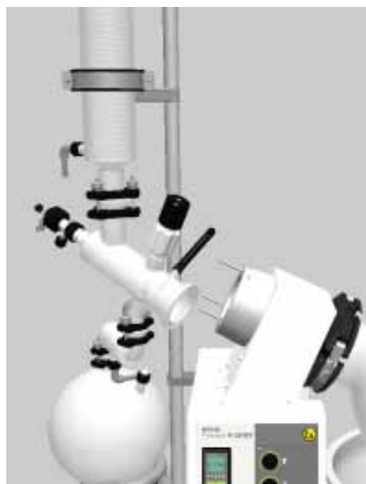
Fig. 31: Replacement of the Vacuum Seal 2
