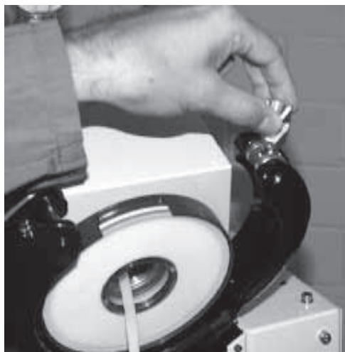
Fig. 14: Adjusting the tension on the closure
