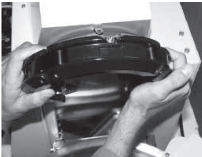
Fig. 25: Assembling the snap flange coupling
