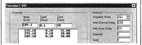
In the above example we have 0.2 sec Dwell times with a 0.02 sec Inter-Channel Delay and a 0.3 sec Inter Scan Delay.
