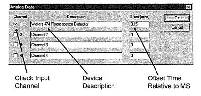
Note that analog data is only acquired while the mass spectrometer is acquiring.
