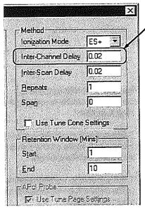
Background: The system monitors one mass (m/z) for a time specified as the dwell time and records a data point for that mass. Before the system can move on and start to monitor the next mass in the list, a short amount of time is needed to reset the electronics and clear the ions from the just measured mass out of the system. This time between the masses listed in a function is called the 'Interchannel Delay'.
