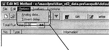
Use these menu items to collect 'Analog Data' such as the voltage output of a UV detector or to use the divert valve for a 'Solvent Delay'.
