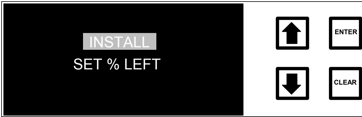
FIGURE 8-13: TUBING INSTALLATION Menu
