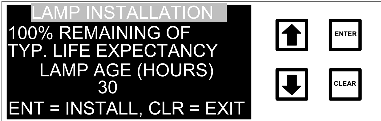
FIGURE 8-12: LAMP Status and INSTALLATION Screen
