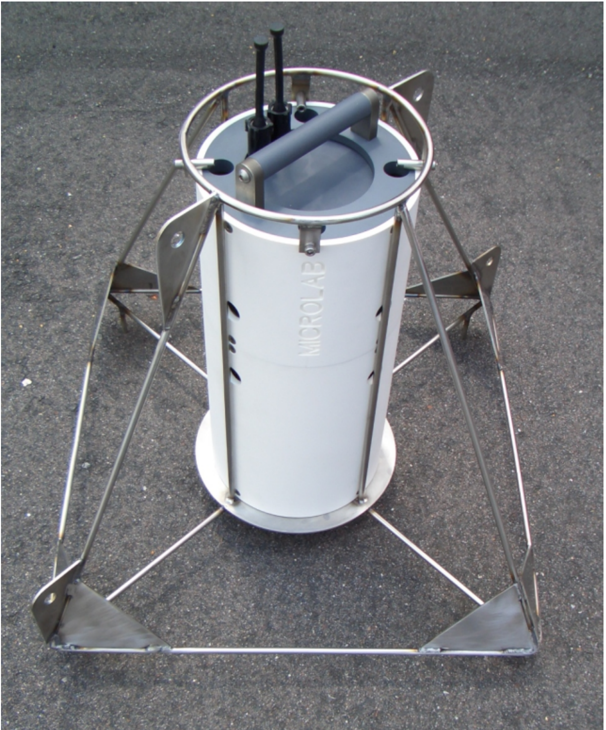
MicroLAB system installed in the bottom deployment frame
