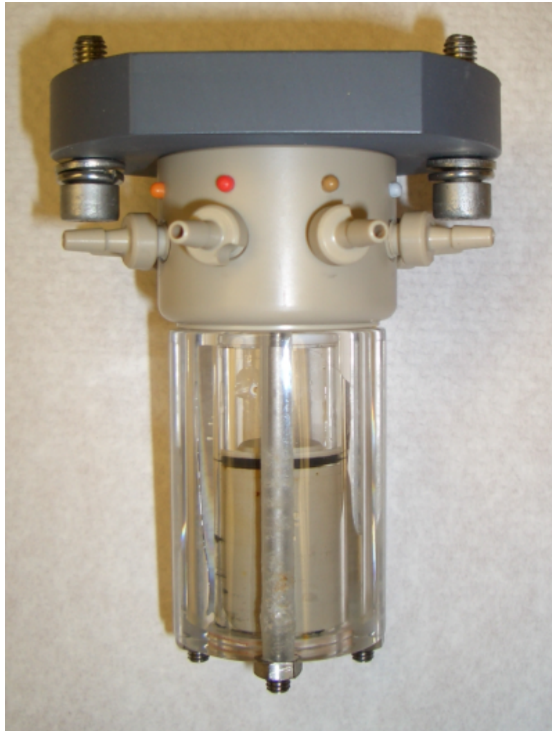
Valve and Syringe Assembly - Spares only. Useful spare for quick turn-around between deployments.
