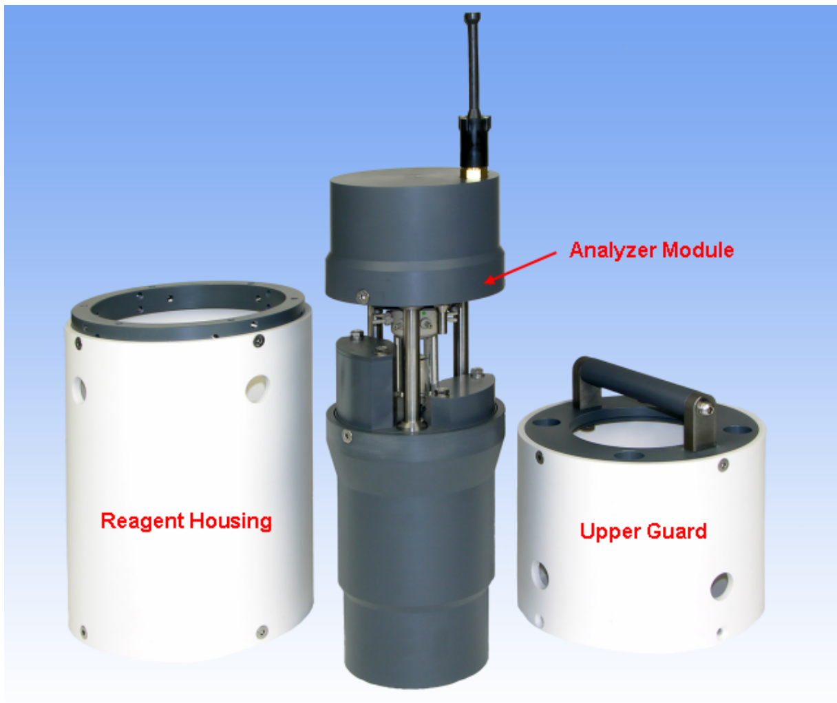
MicroLAB with reagent housing and guard removed
