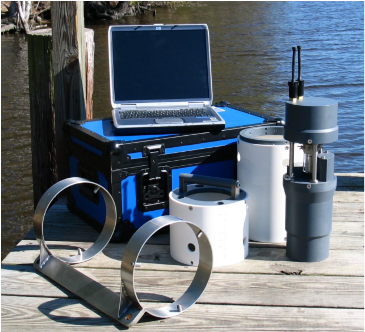
MicroLAB system with the in-line deployment frame in the foreground
