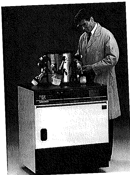
In the manifold drying method, flasks are individually attached to the ports of a drying chamber.
