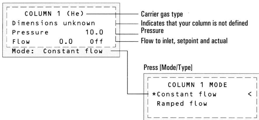
**Figure 39 Column display — Packed or undefined capillary columns**
