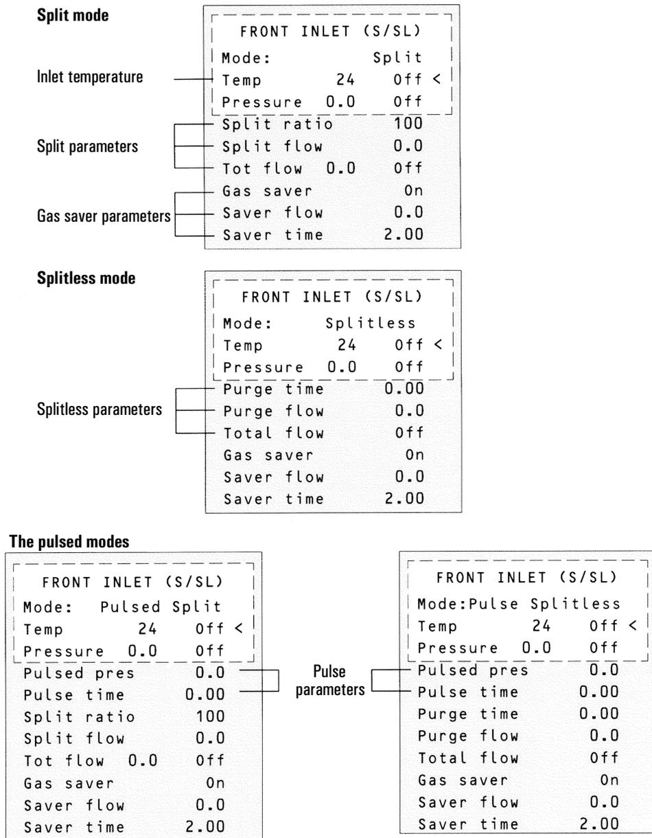
**Figure 6 Control tables for the Split/ Splitless inlet**
