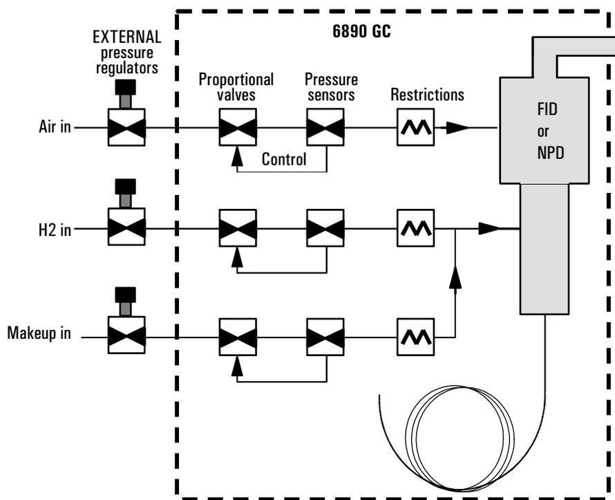
**Figure 7** Internal/external plumbing: FID and NPD *with* EPC
