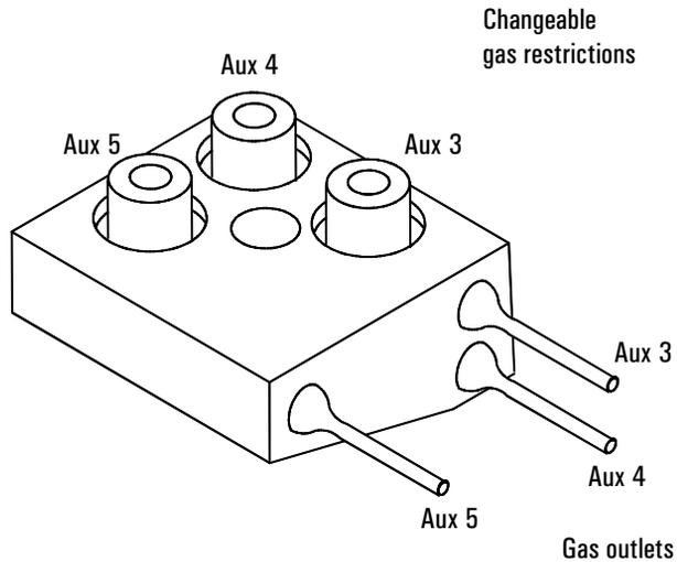
3. Pull the frit to be changed out of the block. Also remove the O-ring that seals it.
