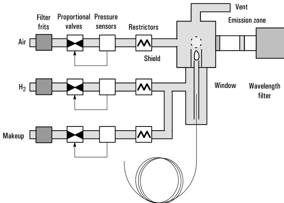
**Figure 10 Internal/external plumbing: FPD with EPC**
