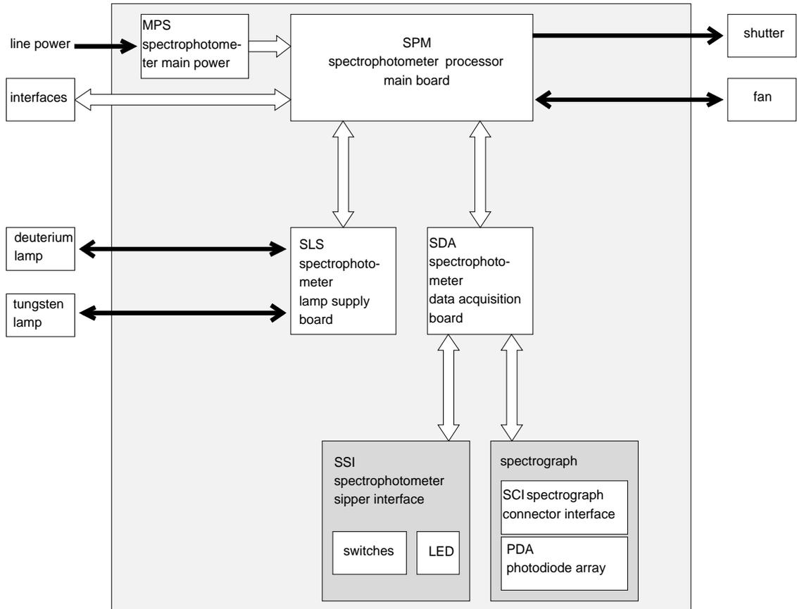
The spectrophotometer includes a spectrograph which utilizes a processor-controlled photodiode array. Several processing steps and hardware boards are required to form spectra from the intensity counts derived from the diode array. Full spectra can be acquired, processed and transmitted every 0.1 s continuously, the only bottleneck being the PC speed. The instrument has its own onboard real-time clock and this allows the instrument to perform a series of time-based accessory control actions and
