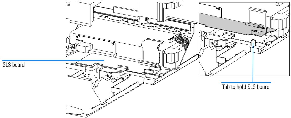
**Replacing the SLS Board**
