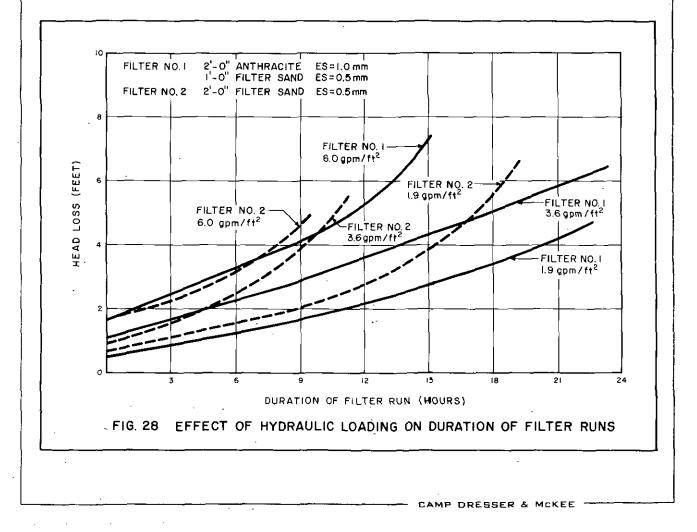
hours. Backwashing of filters was done daily. It is significant to note (*Figure 28*), that the rate of increase of headloss was consistently higher for Filter No. 2 than the rate of increase for Filter No. 1. This may be attributable to the fact that Filter No. 2 had more than twice the height of filter sand than Filter No. 1.
