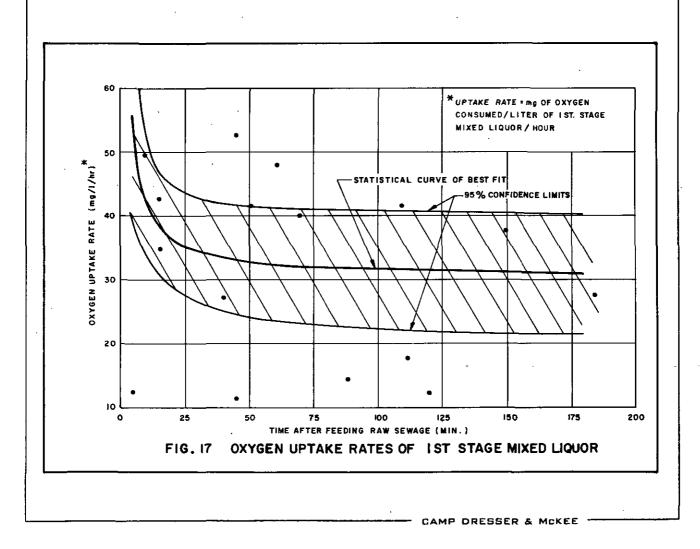
the ammonia removal process occurring in the second stage was not as sensitive to changes in ammonia concentrations as the first stage system was to changes in BOD concentration. Also, in both stages, there was very little decrease in the oxygen uptake rates after about 60 minutes of detention time, indicating that the sample was beginning to approach the endogenous phase.
