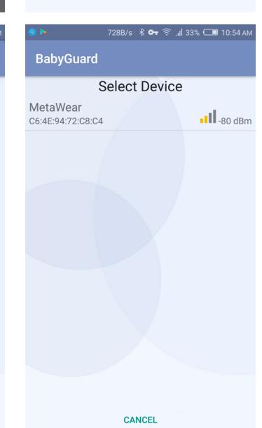
The alarms have also been implemented: once the wearable device's Bluetooth is disconnected, alarm 1 will be triggered, and when temperature is above user defined threshold, the alarm 2 will be triggered.
