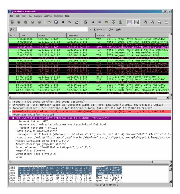
• Since this lab is about Ethernet and ARP, we're not interested in IP or higher layer protocols. So let's change Wireshark's "listing of captured packets" window so that it shows information only about protocols below IP. To have Wireshark do this, select *Analyze->Enabled Protocols*. Then uncheck the IPv4 box and select OK
