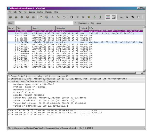
In the example above, the first two frames in the trace contain ARP messages (as does the 6<sup>th</sup> message). The screen shot above corresponds to the trace referenced in footnote 1.
