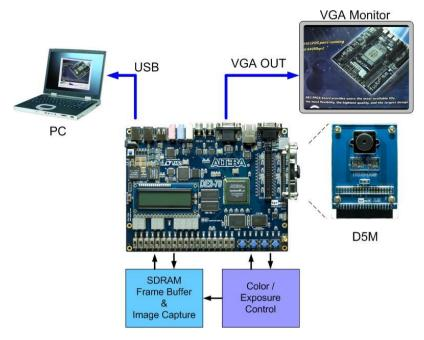
Figure 3-3 The Connection Setup for DE2-70 users
