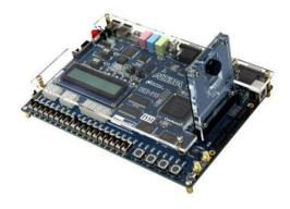
Figure 1-3 Connect the D5M to DE2-115 board's expansion port
