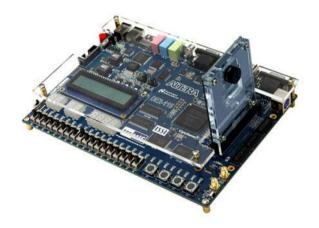
Figure 3-2 The Connection Setup for DE2-115 users
