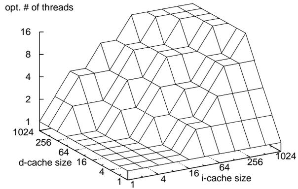
**Figure 7. Optimal Number of Threads for Cache Configuration.**
