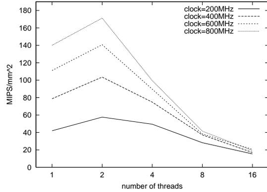
**Figure 6. Performance Depending on Processor Clock Rate and Number of Threads.**
