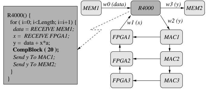
Fig. 9. Inter-core synchronization
