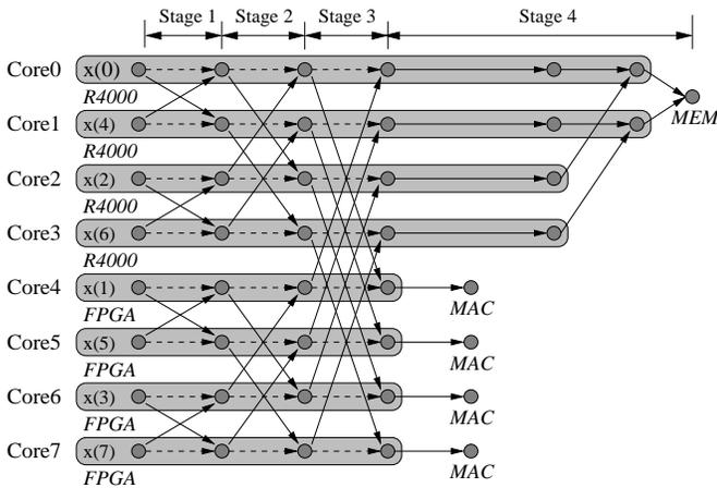
Fig. 12. OFDM mapped to 16 core aSOC model
