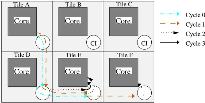
Fig. 3. Pipelined stream communication across multiple communication interfaces
