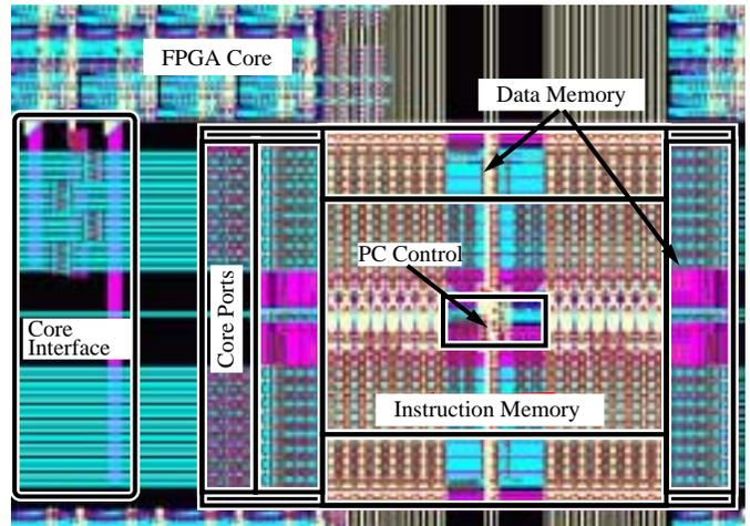
Fig. 14. Layout of FPGA core and communication interface
