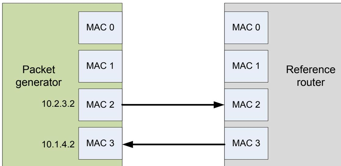
**Figure 8: DE5 NetFPGA Reference router-Packet generator setup**
