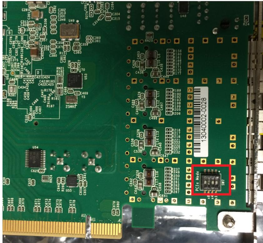
**Figure 2: PCI Express Control DIP Switch**
