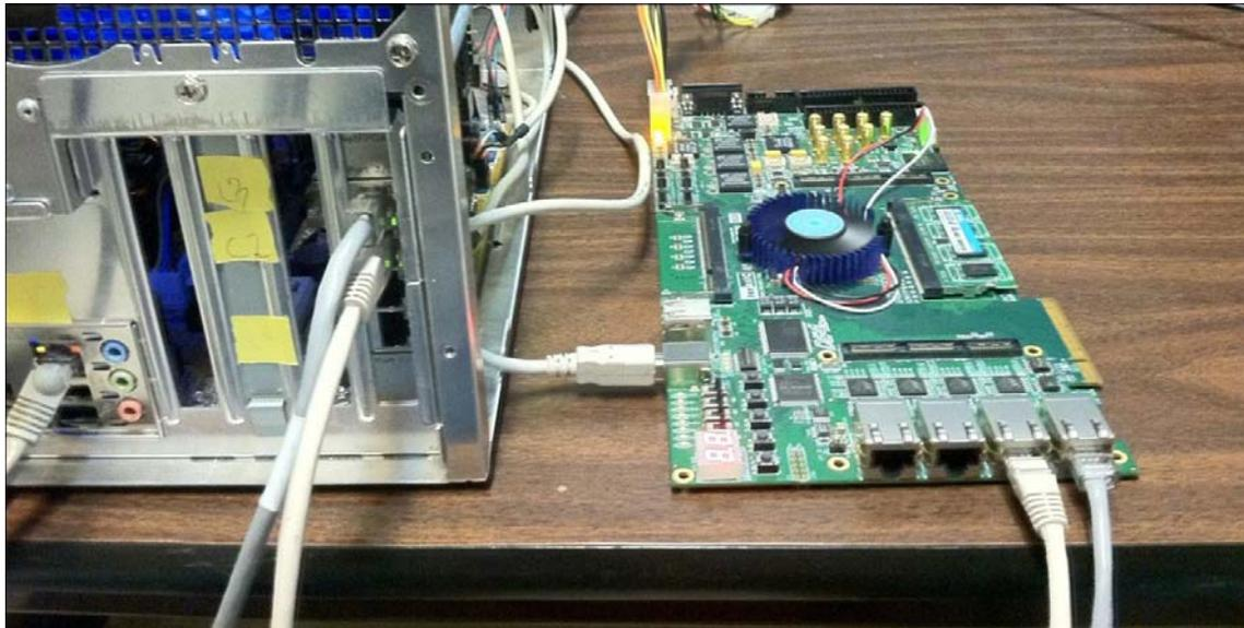
**Figure 17: Test setup with NetFPGA cube and JTAG mode DE4 Reference Router**
