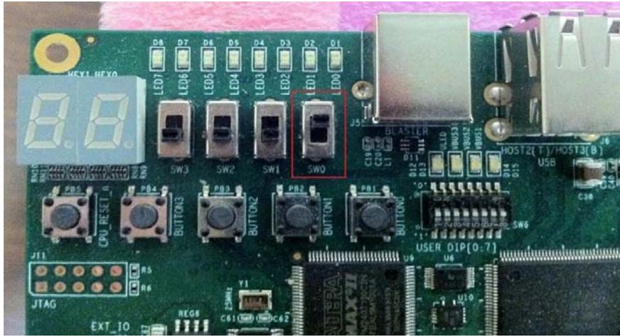
**Figure 2: SW0 switch ON position**
