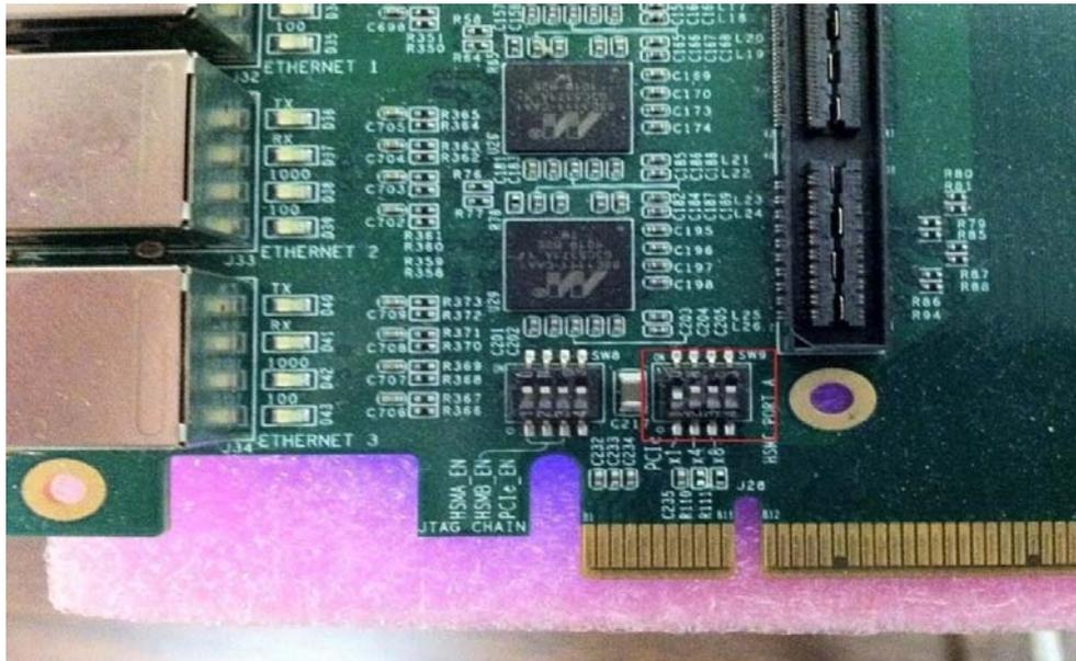
Figure 5: PCI Express Control DIP Switch
