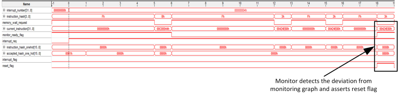
Fig. 4. Attack on processor system, which is detected by hardware monitor.
