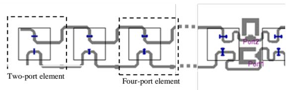
Fig 3. Linear array antenna for elevation plane
