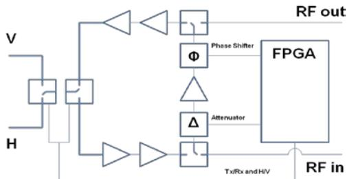
Fig 4. T/R module block diagram
