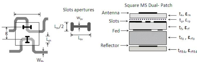
Fig 2. Dual Polarized Patch and stack up
