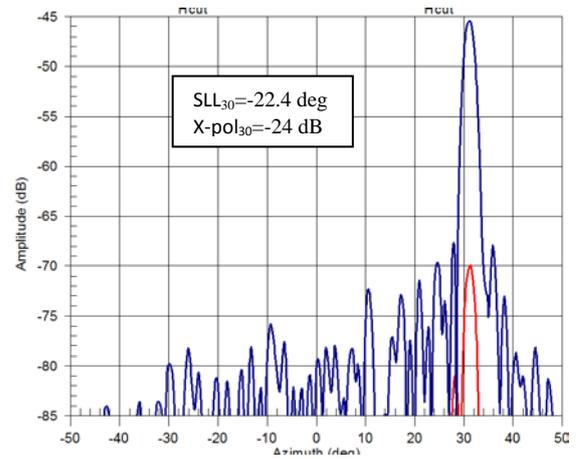
Fig 6. Measured antenna patterns of array 64x32 elements in azimuth plane at 30 deg. a) H-pol (left) and b) V-pol (right)
