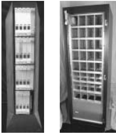
Figure 2: 16-node machine and 128-node chassis.
