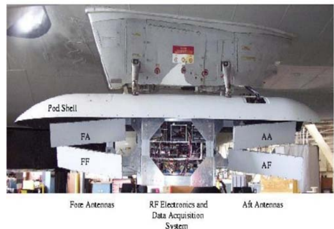
Figure 1. Photograph of DBI installed on the pylon of WP-3D aircraft
