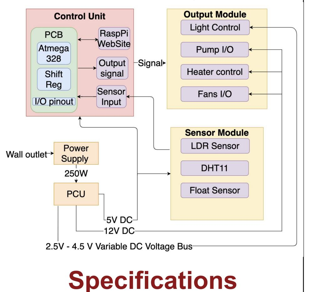
fans, heaters, lights, and water pumps to autonomously grow a plant in the desired conditions. The system is meant to be energy efficient and has the following energy controls..
